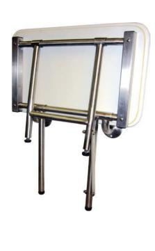
In accordance with ADA requirements, the seat can be raised and lowered with less than 5 pounds of force. Mounting bracket provides smooth, uniform resistance. Positive friction allows the seat to remain securely in the raised position preventing accidental lowering. When installed correctly CSI Shower seats will support a static load of in excess of 400 lbs.
